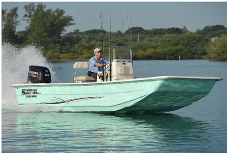
**V-hull** - V bottom boats have a V shape angled bottom, which is called the deadrise angle. The flatter shape of the deadrise the hull will plane with less power but will pound more in the waves. So, the greater the angle the more horsepower required to plane, but the hull will be better suited for rougher weather. The most popular styles of this hull design are: Ocean Racing Motor Boats, offshore sport fishing boats.
